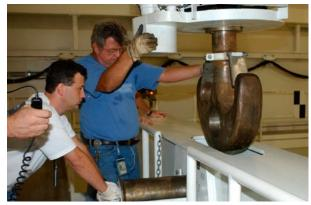
Technicians prepare to install a huge locking pin through the spreader bar and crane hook used to rotate the payload canister in the CRF.
